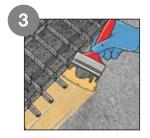
Apply a thin coat of the mixed material on the old concrete surface with the help of a brush, spreader or roller. Allow it to cure for 3 - 4 hour.
