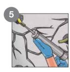
When the material comes out of the other nozzle, it indicates that the cavity is completely filled.
