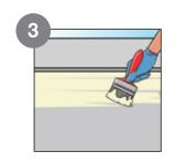
Thoroughly mix Lapox® Lacrete resin and hardener in a 1:0.5 ratio, and apply the waterproofing coating on terrace.
