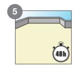
For optimum results, allow the system to cure for a minimum of 48-hour.
