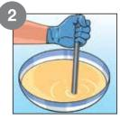
Thoroughly mix Lapox® Lacrete resin and hardener, in a 1:0.5 ratio, in a disposable bowl.
