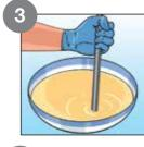
Thoroughly mix Lapox® Lacrete resin and hardener, in a 1:0.5 ratio, with 7 - 8 parts of Quartz Sand no. 10.
