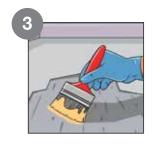
Apply the mixed material in a thin, uniform layer on the substrate with the help of a brush, spreader or roller.
