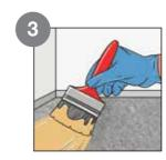
Using a brush, roller or spreader, apply the mixed material in a thin, uniform layer on the substrate. This will act as a primer.
