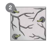
Insert PVC nozzles at the two ends of the cracks. Fix them well using Lapox® Ultraseal (epoxy putty).
