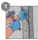
Widen the crack by making a 'V' groove and clean any dust or loose concrete using compressed air or any other suitable means. In case of potholes, loosen the concrete and clean.
