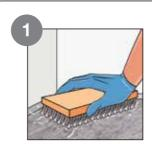
Ensure that the concrete surface is dry, clean and free of contaminants such as oil and grease. Remove loose particles and dust using a wire brush.
