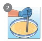
Thoroughly mix Lapox® Lacrete resin and hardener, in a 1:0.5 ratio, with 5 - 6 parts of Quartz Sand no. 10.
