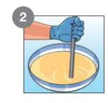
Thoroughly mix Lapox® Lacrete resin and hardener, in a 1:0.5 ratio, in a disposable bowl.
