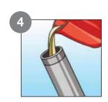
Fill the mixed material in an injection-grouting gun and inject it in the nozzle at a pressure of 7 - 8 bar.
