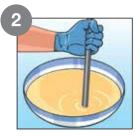
For the primer coat, thoroughly mix Lapox® Lacrete resin and hardener, in a 1:0.5 ratio, in a disposable bowl.
