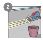
Check for hollow portions and major cracks and fill them with mortar mixed with Lapox® Lacrete. Fill the wall to floor joints (fillets) with the same mortar.
