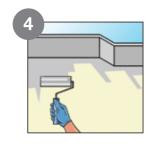
Protect the Lapox® Lacrete waterproofing coating by applying Lapox® Procoat, an UV resistant coating.
