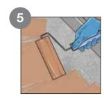
Apply the second waterproofing coat or screed 5 - 6 hour after preparing the angle fillet.
