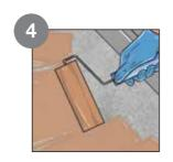
For application of the screed, thoroughly mix Lapox® Lacrete resin and hardener, in a 1:0.5 ratio, with 4 - 5 parts of Quartz Sand no. 10. Thoroughly mix all the ingredients with a trowel to achieve homogeneous consistency. Pour the mixed material on the concrete.
