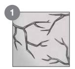
Ensure that the concrete surface with cracks is clean and dry. Remove any loose concrete.
