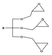
Advantages Extremely low moisture absorption Non-volatile and low odour Provides good flexibility and impact resistance to epoxy systems Superior electrical properties
