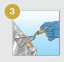
Apply the mixed material using a brush or a spatula on the surface to be adhered within its pot life time.
